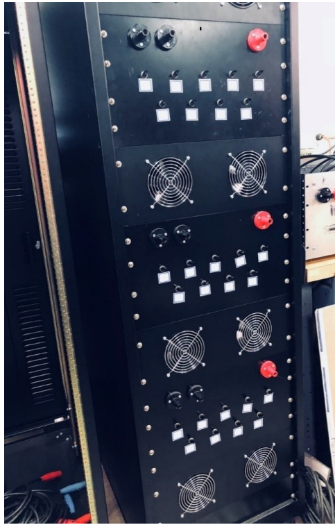
Figure 3: The load resistance hardware
