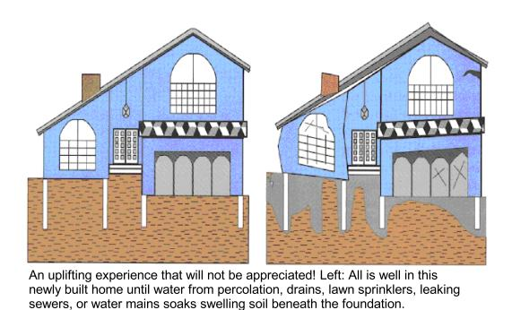
Right: With time, expanding soils exert several tons per square foot of pressure on the foundation and shallow pilings. Without remedial measures, the house will actually become deformed, and shatter masonry and windows. Remedies vary from mere maintenance that keeps drainage away from the house to expensive reconstruction of foundations. Prior site planning that takes geology into account is always preferable to dealing with problems after a structure is built. From AIPG (1993).
