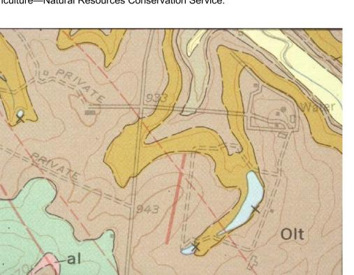
Geologic map showing existing ponds located below the seepage zone in the illustration above. Ponds should be constructed so that the springs or seeps will always be above the level of the pond surface. Illustration by Paul Howell, U.S. Department of Agriculture—Natural Resources Conservation Service.
