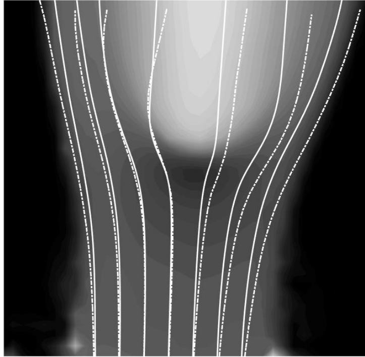
Figure 6.1: Streamline effect from a single (solid) and interacting (dashed) triple flame. The color scale represents the velocity magnitude of the single triple flame
