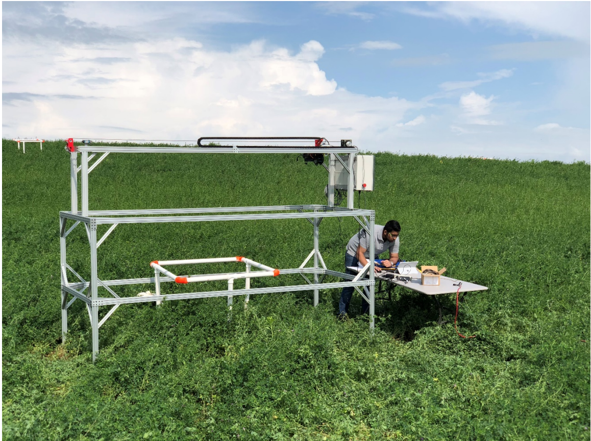
Figure 4-2: Modeling the alfalfa using the linear motion system over a quadrat
