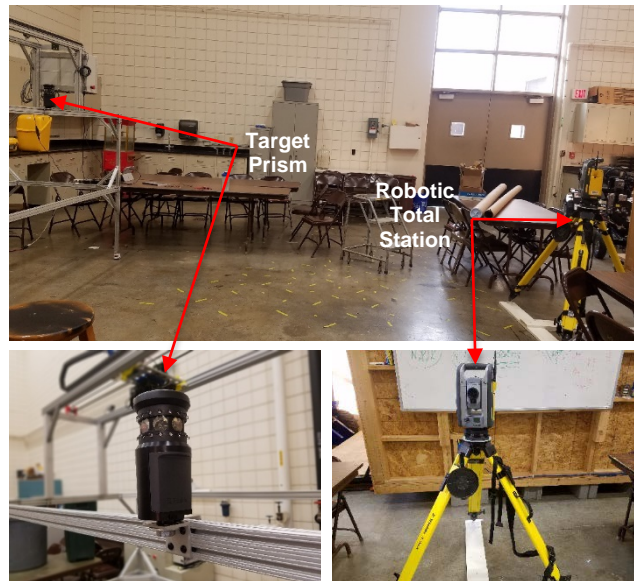
Figure 2-6: Validation of the linear motion system performance using a robotic total station and target prism.
