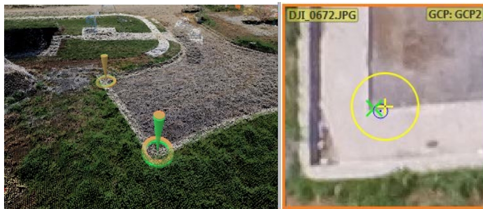
Figure 2.6 Marking a GCP
