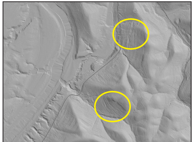
Figure 7. LiDAR hillshade exhibiting hummocky slopes and roughness. Although these slopes may be creeping, the roughness is probably an artifact of forested slopes, aspect, and geology.
