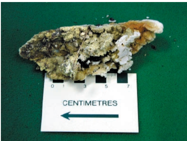
Figure 30. Secondary sulfates copiapite and melanterite derived from retaining-wall drain tiles at rear of middle school.
