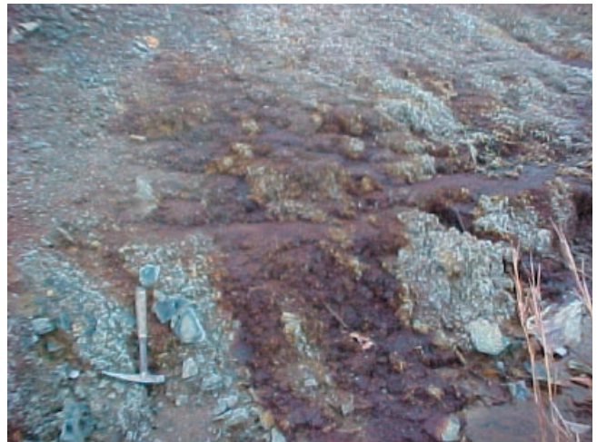
Figure 7. Pyrite oxidation, iron oxide, and sulfate staining and precipitate in the Chattanooga Shale at the middle school.
