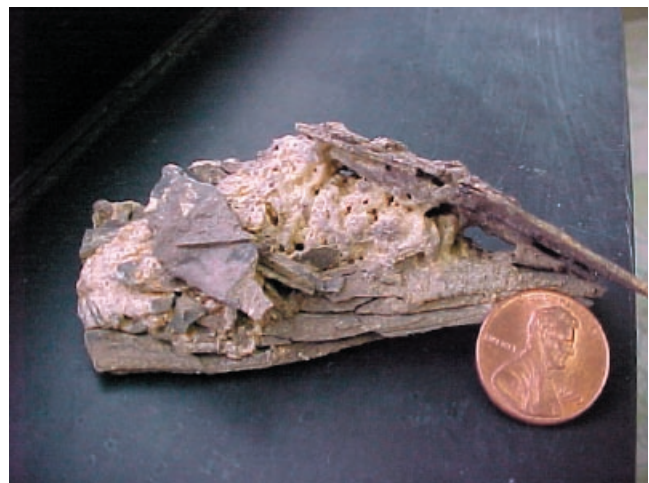
Figure 31. Evidence of heaving by growth of secondary sulfate copiapite in the Chattanooga Shale.
