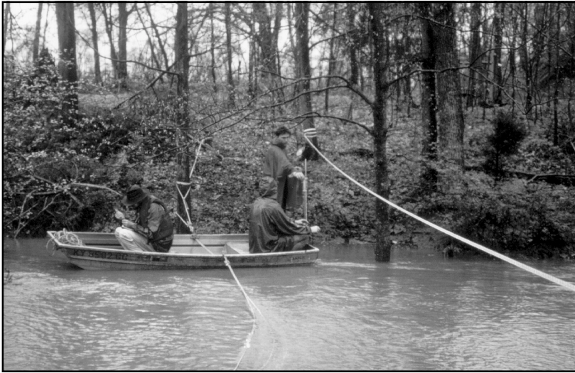
Figure 6. Discharge measurements being made at Pleasant Grove Spring during the May 1993 high-flow event.
