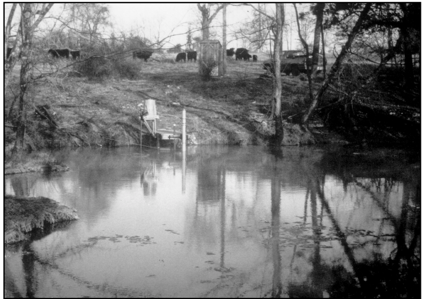
Figure 5. Instrumentation, supported by a pier, in the mouth of Pleasant Grove Spring. Storage shed housing data loggers and other equipment is in the background.
