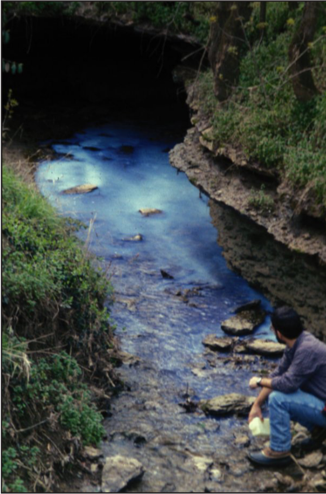
Figure 6. Optical brightener (Tinopal CBS-X) being poured into a sinking stream cave entrance, Bourbon County. Photo by J.C. Currens.
