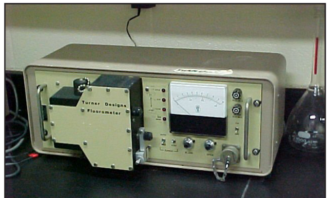
Figure 9. Analog filter fluorometer. The instrument shown can be configured for Fluorescein and Rhodamine WT. Photo by J.C. Currens.
