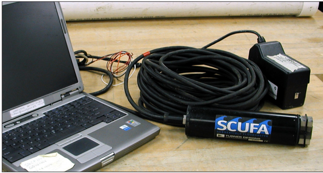
Figure 11. Submersible fluorometer with 30 m of cable. The device requires a 12-volt auxiliary power supply and is programmed and downloaded using software installed on a laptop computer. Photo by Collie Rulo, Kentucky Geological Survey.
