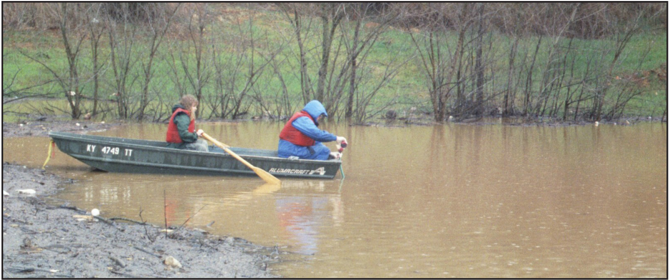
Figure 7. Introduction of a quantitative trace into an inundated swallow hole, Hardin County. The water was over 5 m deep and the boat was positioned using landmarks. A garden hose was inserted into the swallow hole, and a funnel was used to pour the Rhodamine WT into the hose. The total head in the swallow hole was less than at the surface, and the dye was quickly drawn down the hose. Photo by David Lutz.
