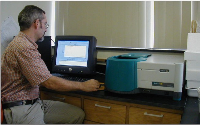
Figure 10. Synchronous scan fluorescence spectrophotometer. The system is entirely digital. Photo by J.C. Currens.
