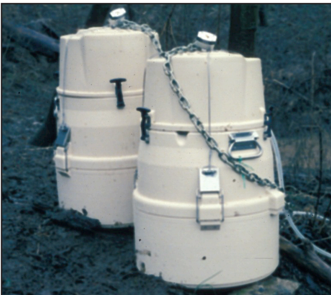
Figure 8. Automatic water-sampling machines set up to collect two 24-bottle series of samples. Photo by J.C. Currens.
