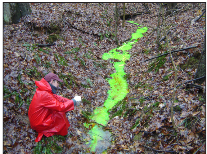
Figure 5. Textbook example of Sodium Fluorescein injection into a sinking stream. The dark object at the distant terminus of the dye is the swallow hole. Fort Knox Military Reservation. Photo by David Lutz.
