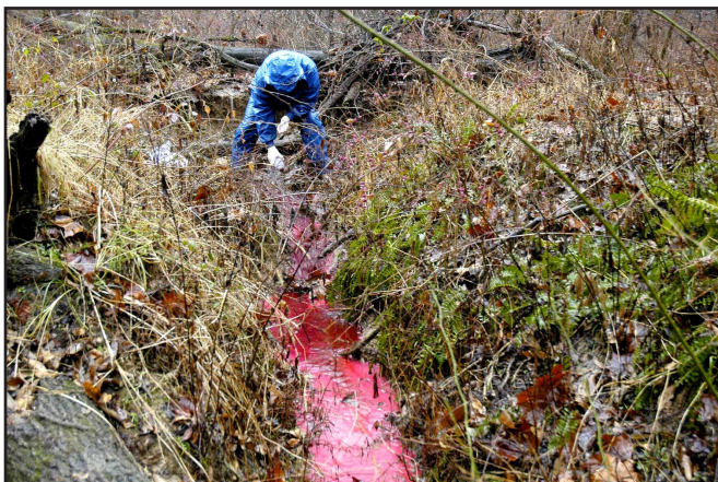
Figure 4. Sulforhodamine B being poured into a sinking stream in Hardin County. Notice the stance of the researcher above the water, with feet away from the tracer. The wind direction should be toward the camera. Photo by David Lutz.
