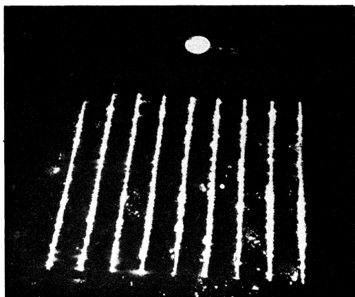
Fig. 2—Lines of marble dust and soil stress transducer placed within the profile.
