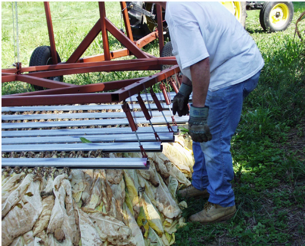
Figure 5. Manually connecting piston-type attachment devices on the carrying frame to the ends of filled rails lying on the ground.
