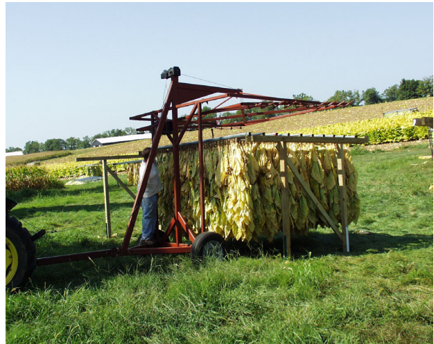
Figure 7. Retriever/transporter placing rails of tobacco on a field curing structure.
