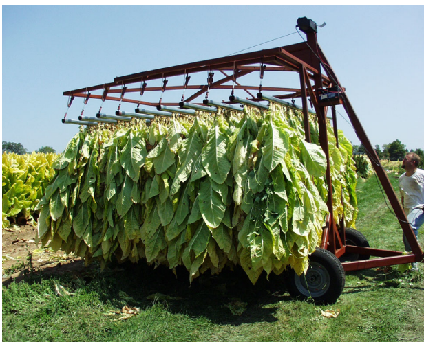
Figure 6. Retriever/transporter with load hoisted for transport.
