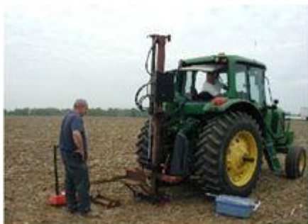
Figure 5. Multi-probe soil cone penetrometer (left) and nuclear density testing machine (right).
