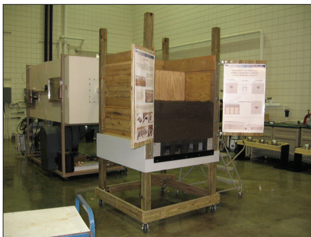
Figure 3. Biofilter used for preliminary pressure drop tests.
