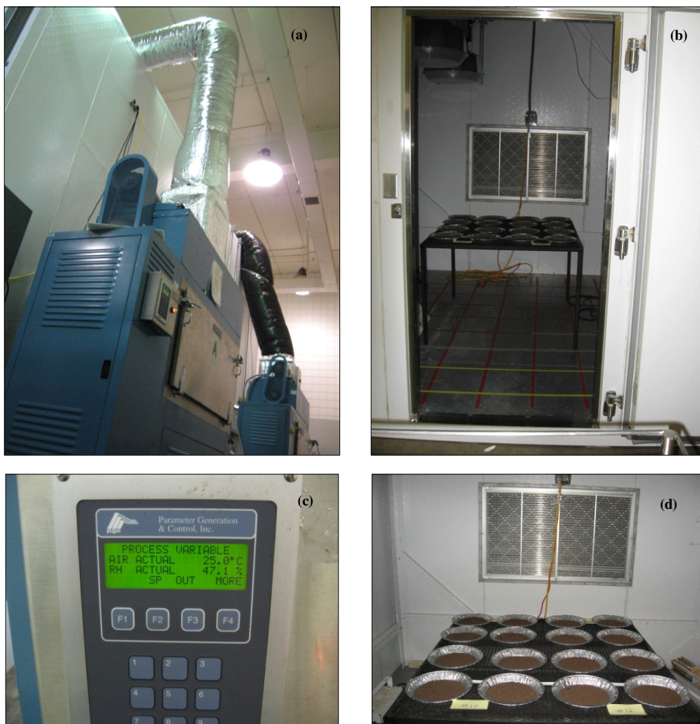
Figure 1. Environmental chamber controlled for temperature and relative humidity (Parameter Generation and Control, Black Mountain, N.C.): (a) rear view, (b) front view with door open, (c) input parameter control display, and (d) interior with 16 sieved compost samples.
