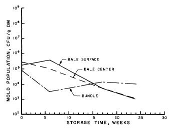
Fig. 2—Mold population (colony forming units/g dry matter) of bales and bundles as a function of time of storage.
