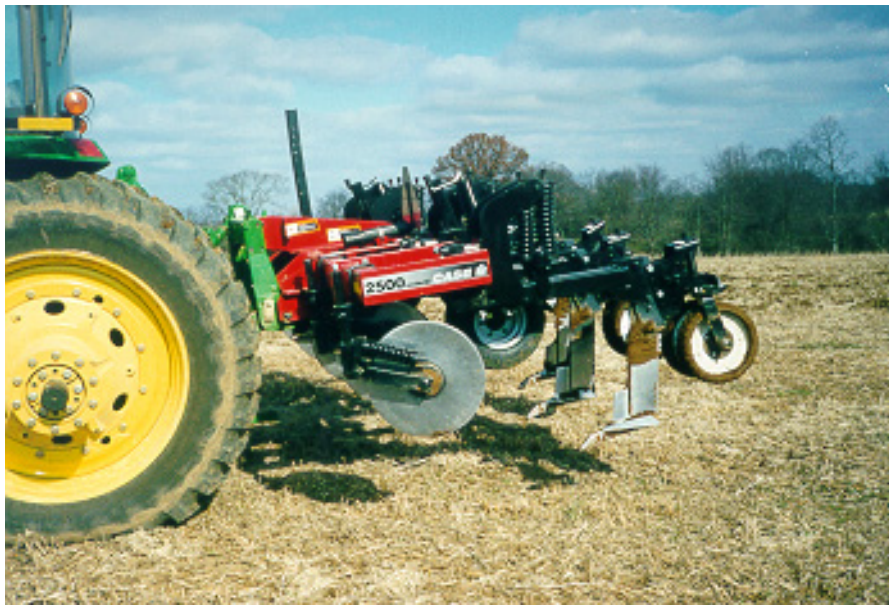
Figure 2. Case-IH Ecolo-til 2500 subsoiler (2000 model) with five shanks spaced at 76 cm (30 in.) with a maximum tillage depth of 40 cm (16 in.).
