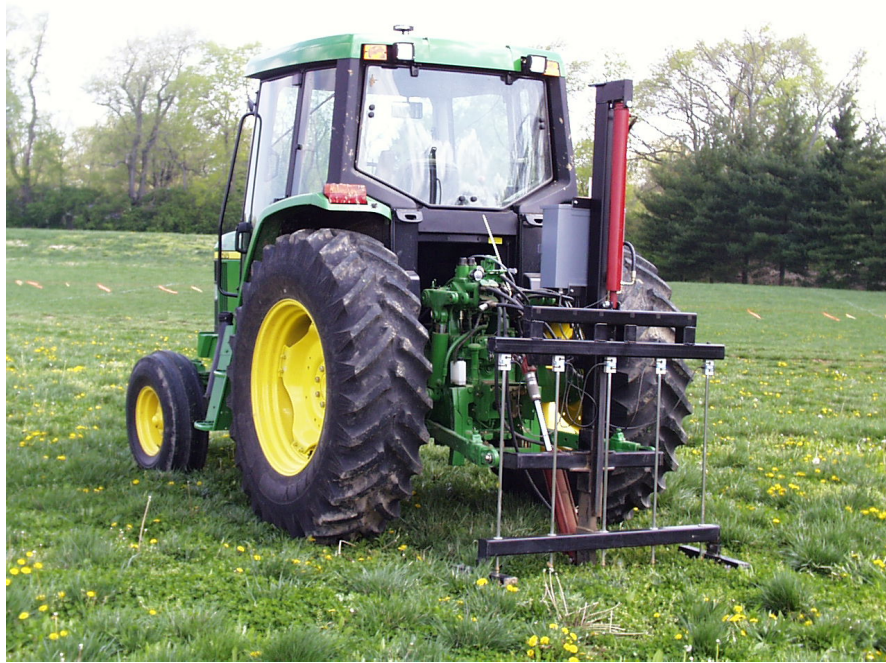
Figure 1. Tractor-mounted, multi-probe recording soil cone penetrometer equipped with DGPS.
