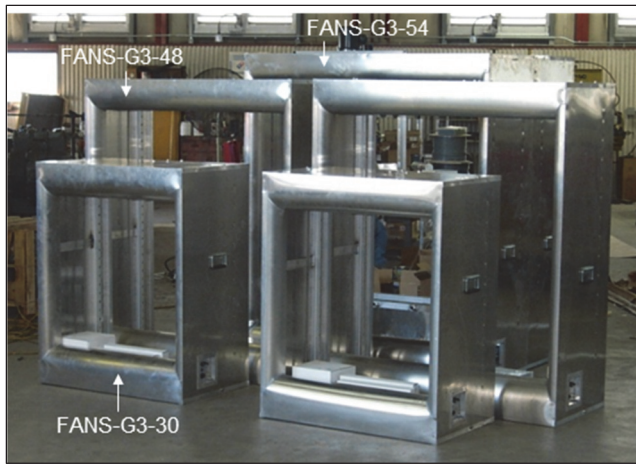
Figure 1. Three models of third-generation FANS (FANS-G3) units for in situ volumetric airflow measurements on 76 cm (30 in.), 122 cm (48 in.), and 137 cm (54 in.) size ventilation fans.
