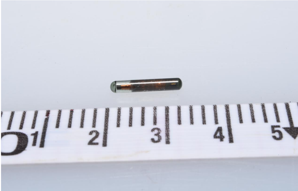
Figure 3.1 Passive Integrated Transponder (PIT) Tag. An 134.2 kHz 12.5 mm passive integrated transponder (PIT) tag used to subcutaneously mark snakes.
