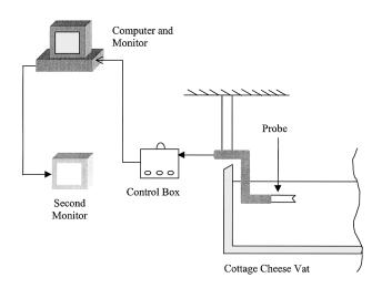
Figure 1–Schematic of the cottage cheese culture monitoring system installed at Winchester Farms Dairy.
