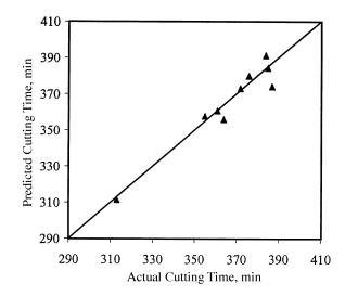
Figure 6–Plot of actual and predicted cutting times for the data collected March through May 1998 using the algorithm  $T_{cut} = T_{max} + \beta_2 S$ .
