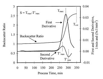
Figure 3–Backscatter ratio profile with the corresponding first and second derivative curves with curve parameters  $T_{cut}$ ,  $T_{max}$ ,  $T'_{max}$ , and  $T'_{min}$  identified. The second derivative curve has been scaled for emphasis.
