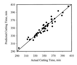
Figure 4–Plot of actual and predicted cutting times for the data collected July through October 1997 using the algorithm  $T_{cut} = T_{max} + \beta_2 S$ .
