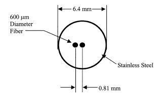
Figure 2–Schematic of the probe tip used to monitor the light backscatter during the coagulation of cottage cheese. The optical fiber located in the center emits light into the milk and the fiber located 0.81 mm from the center transmits the light scattered back to a photodetector.
