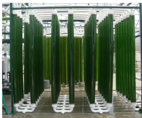
Fig. 1 CAD image showing PBR design and photograph of the PBR installed in a greenhouse
