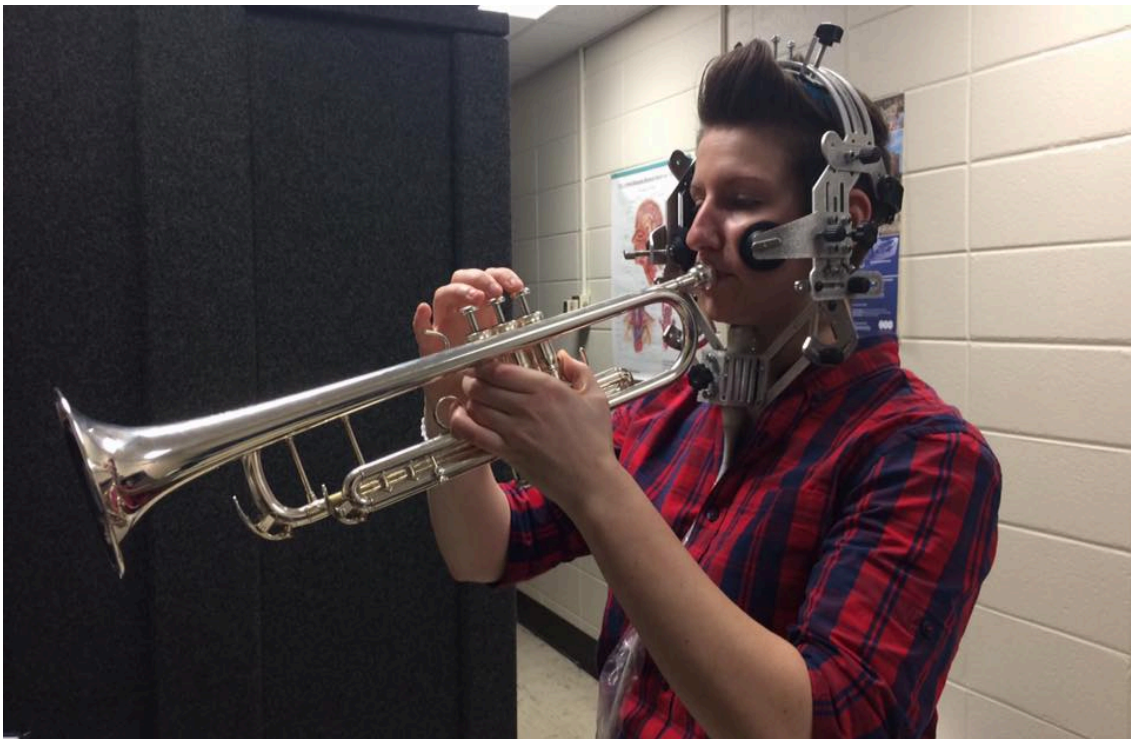
Figure 4.5 – Author playing trumpet with headset. Transducer attached under chin.
