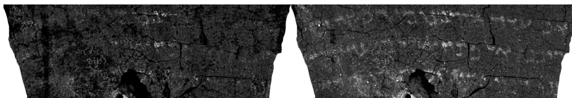
Fig. 7. The effect of directional texturing to improve ink response. (Left) Intersection of the mesh with the volume. (Right) Directional texturing with a neighborhood radius of 7 voxels.
