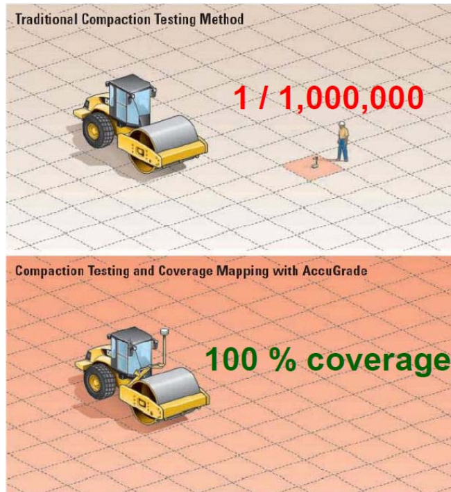
Figure 7.2: Intelligent Compaction Results (Willoughby 2014)
