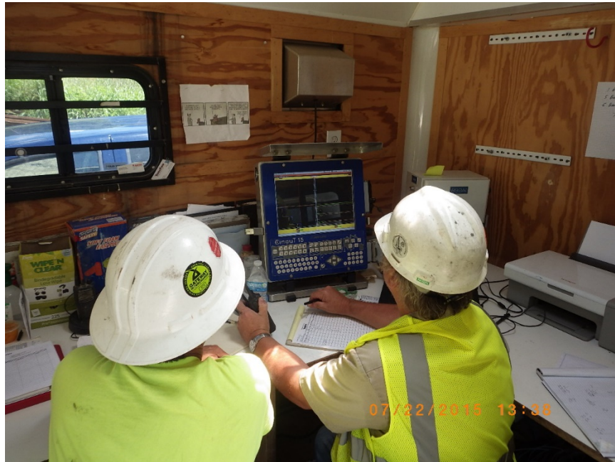
Figure 18. Automated Grouting and Data Collection System Operation
