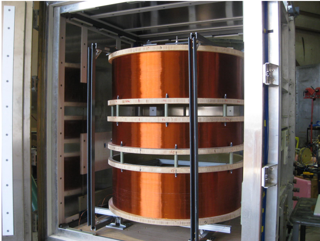
Figure 4.12: Double-gapped solenoid inside shield. The two vertical struts in the foreground, resting on the top of the B_0 frame, are rectangular fiberglass frames which support the spin-flipping B_1 coils.
