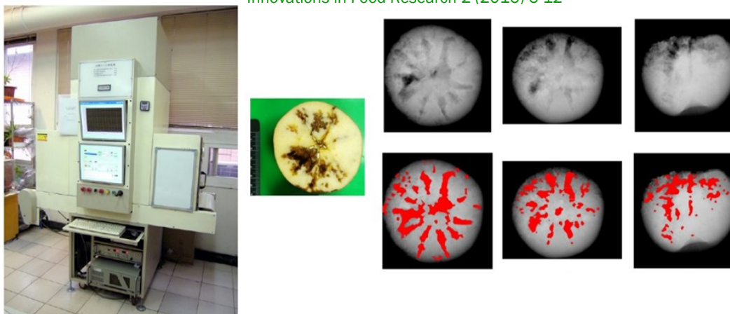
Figure 5. The photograph of automatic x-ray scanner (left), x-ray images of the apple scanned and the segmentation results (right). Source: Chuang et al. 2011
