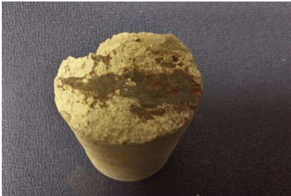
Figure 7. Corrosion at the Level of the Steel, Hardin County
