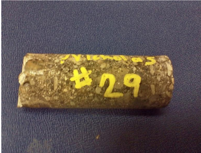
Figure 9. Results of Core Testing with Silver Nitrate Solution for Chlorides
