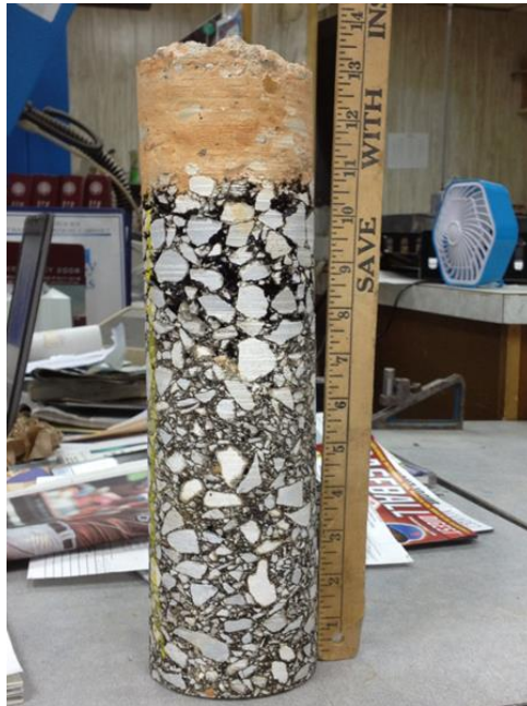
Figure 2 Pavement core obtained from the Pulaski County KY 80 Project. (Photograph courtesy of Neil Ryan, Mount Carmel Stabilization Group)
