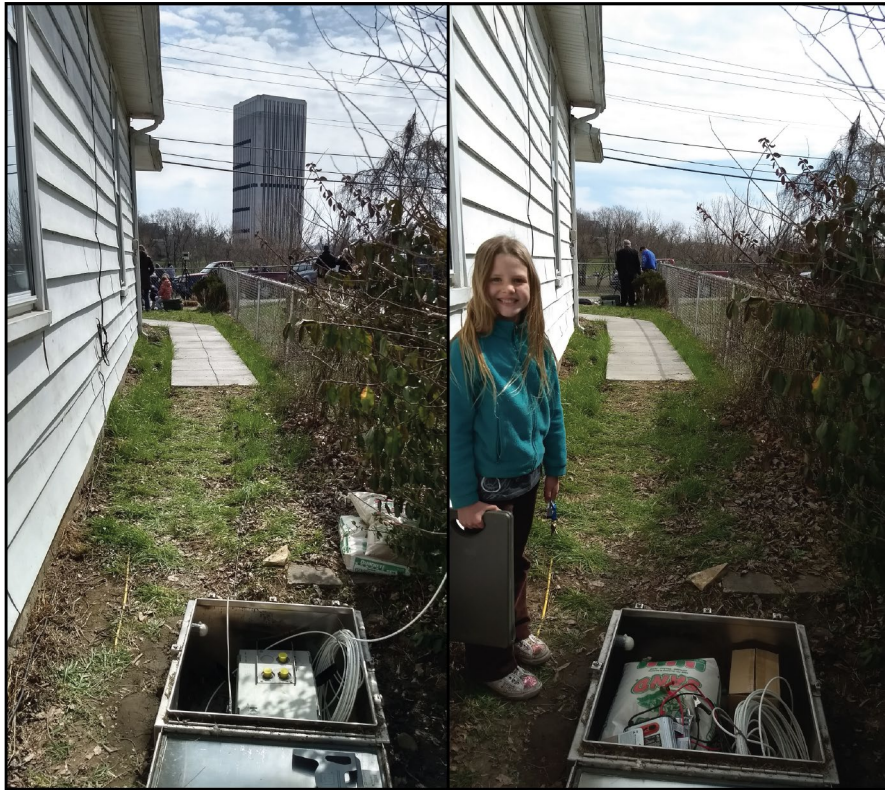
Figure 10. (Left) Capital Plaza Tower from the location of station CPT1 shortly before the implosion. (Right) The same view, shortly after the building's demolition, with a student observer next to the instrument. Photos by Seth Carpenter.
