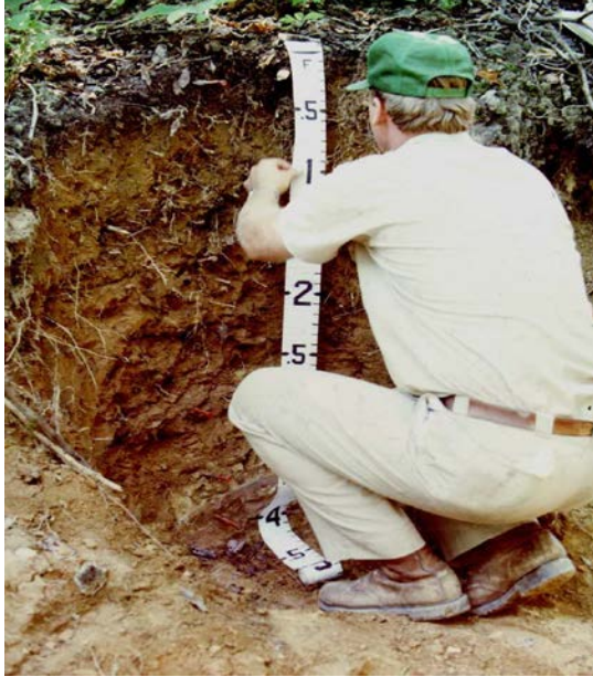
Fig. 9. Taking accurate soil horizon and depth measurements are an important part of describing a soil.
