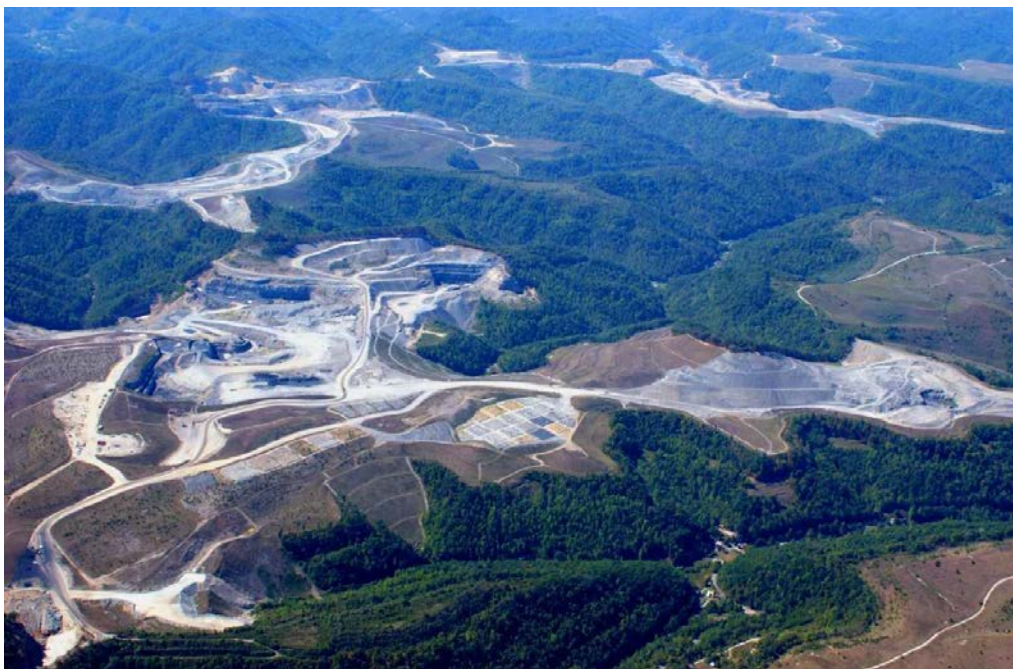
Fig. 110. An aerial view of coal mining using the mountain top removal approach in the Eastern Coalfields (Chris Barton)
