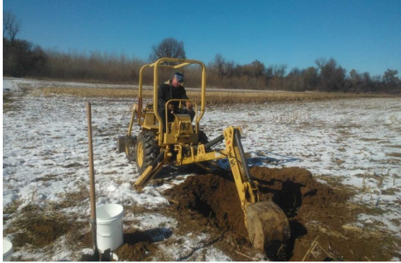
Fig. 7. Excavating a soil pit with a backhoe is always the easiest way to describe a soil regardless of weather conditions.
