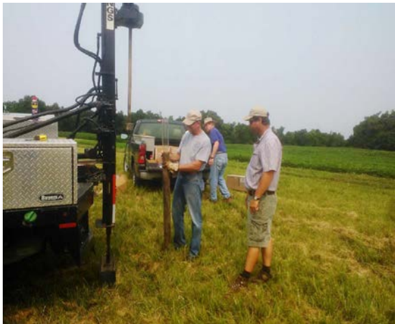
Fig. 5. Truck mounted hydraulic probes have considerably facilitated soil sampling in the last 20 years.
