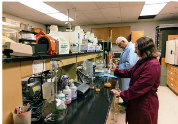
Fig. 15. Soil samples are analyzed in the laboratory to provide additional characterization data for accurate soil identification and classification.
