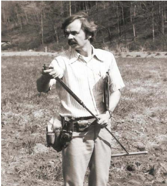
Fig. 3. A push probe can provide some preliminary soil information in soil areas without gravel or rock fragments.
