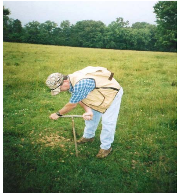
Fig. 4. A bucket auger is more efficient for preliminary surveys of inaccessible or fragmental soils.
