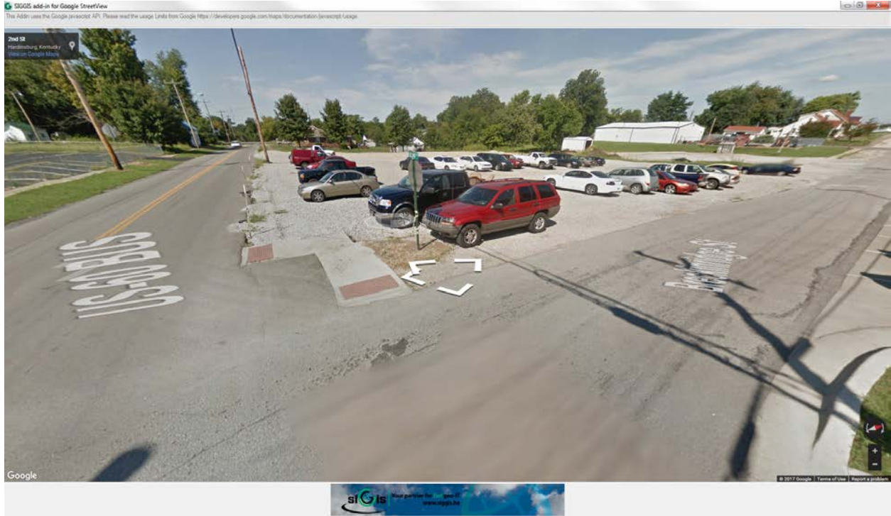
Figure 25: Two Ramps with Detectable Warnings (Rampcorner=1, Ramptype=2, RampDW=1)
