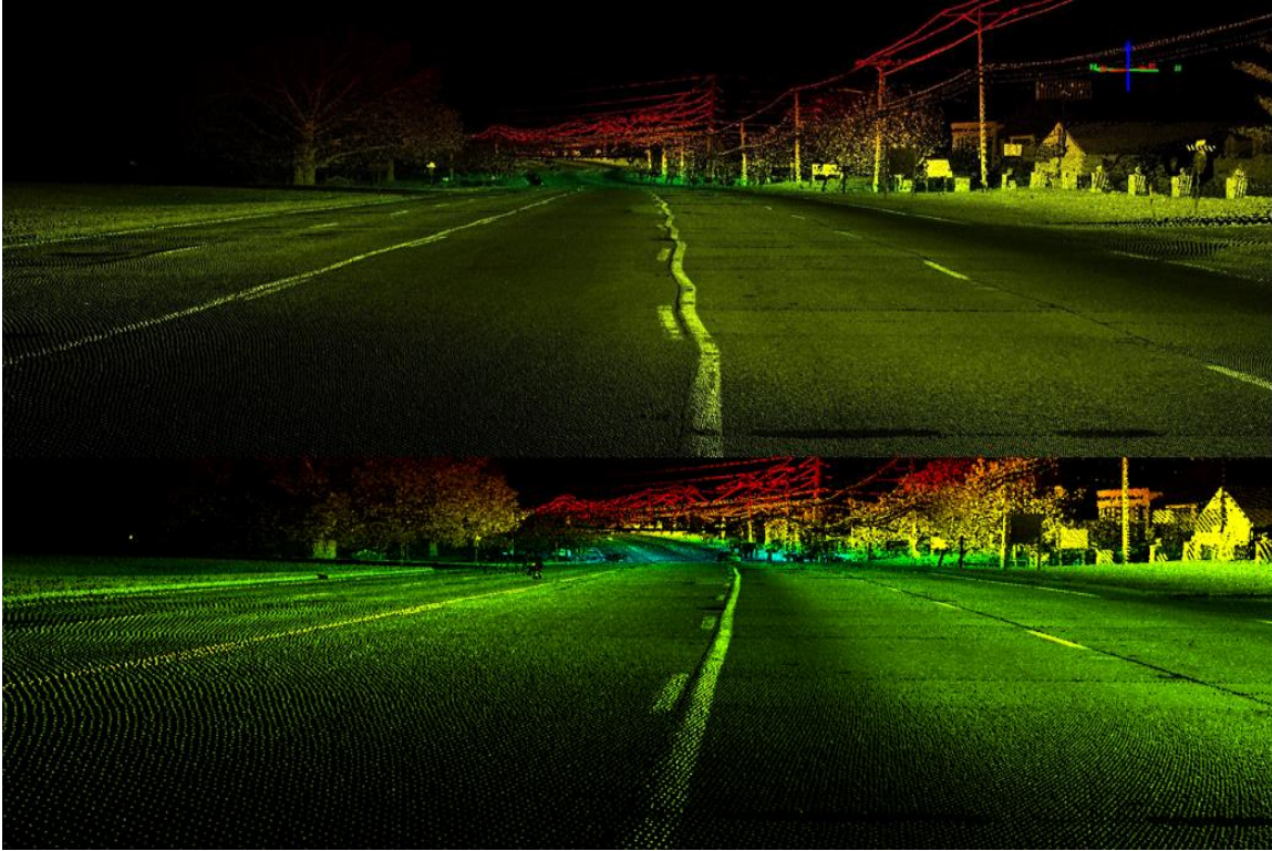
Figure 16 Effect of G4 solar storm on mobile Lidar data
