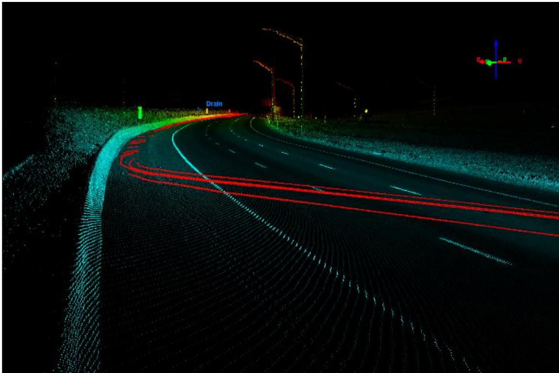
Figure 6 Water flows along barrier wall and returns to roadway surface
