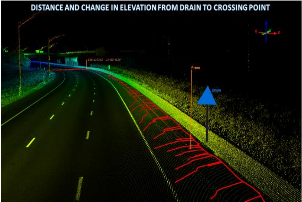
Figure 5 Water flow analysis depicting water flow paths
