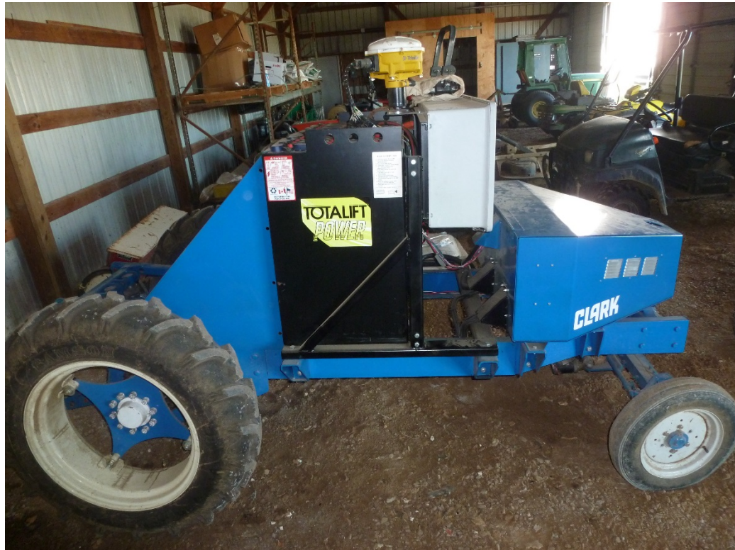
Figure 4-1 Fully electric autonomous tractor version 2.0
