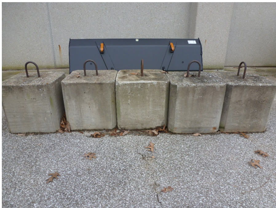
Figure 4-9 Concrete weights for the sled
