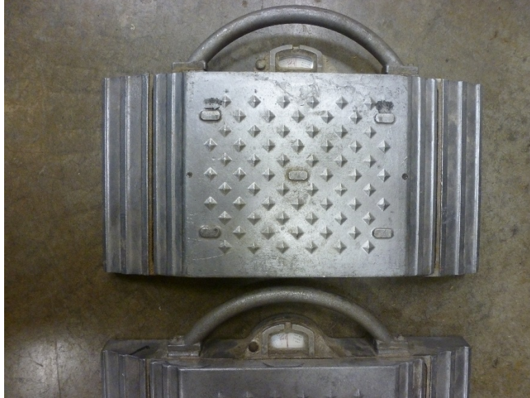
Figure 4-10 Wheel scales with Vernier measurement
