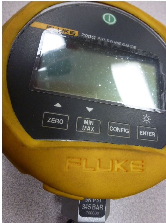
Figure 4-17 Fluke 700G30 pressure gauge
