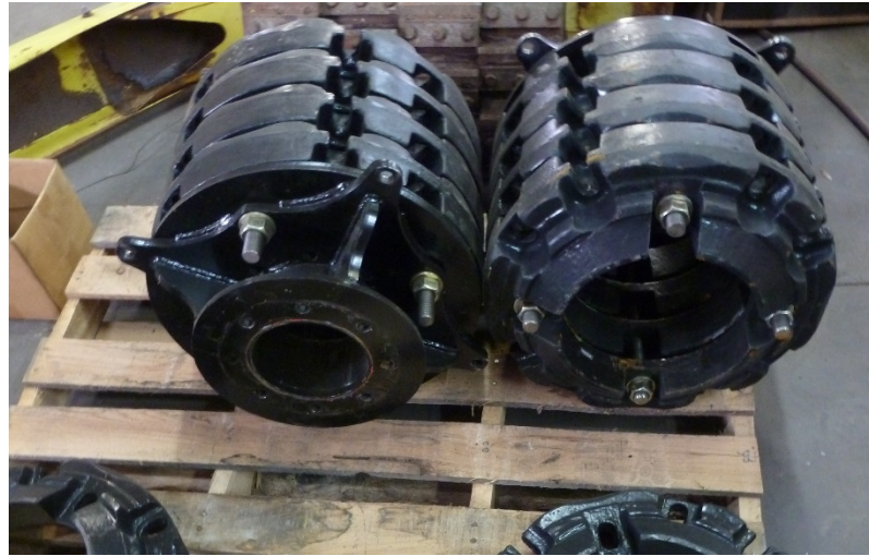
Figure 4-5 Custom wheel centers with ballasts
