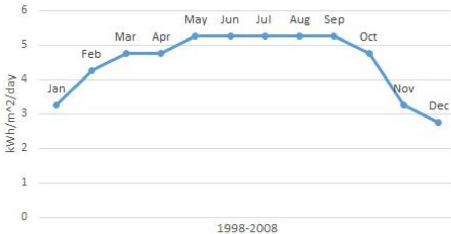
Figure 5-13 NREL solar photovoltaic resource potential for KY
