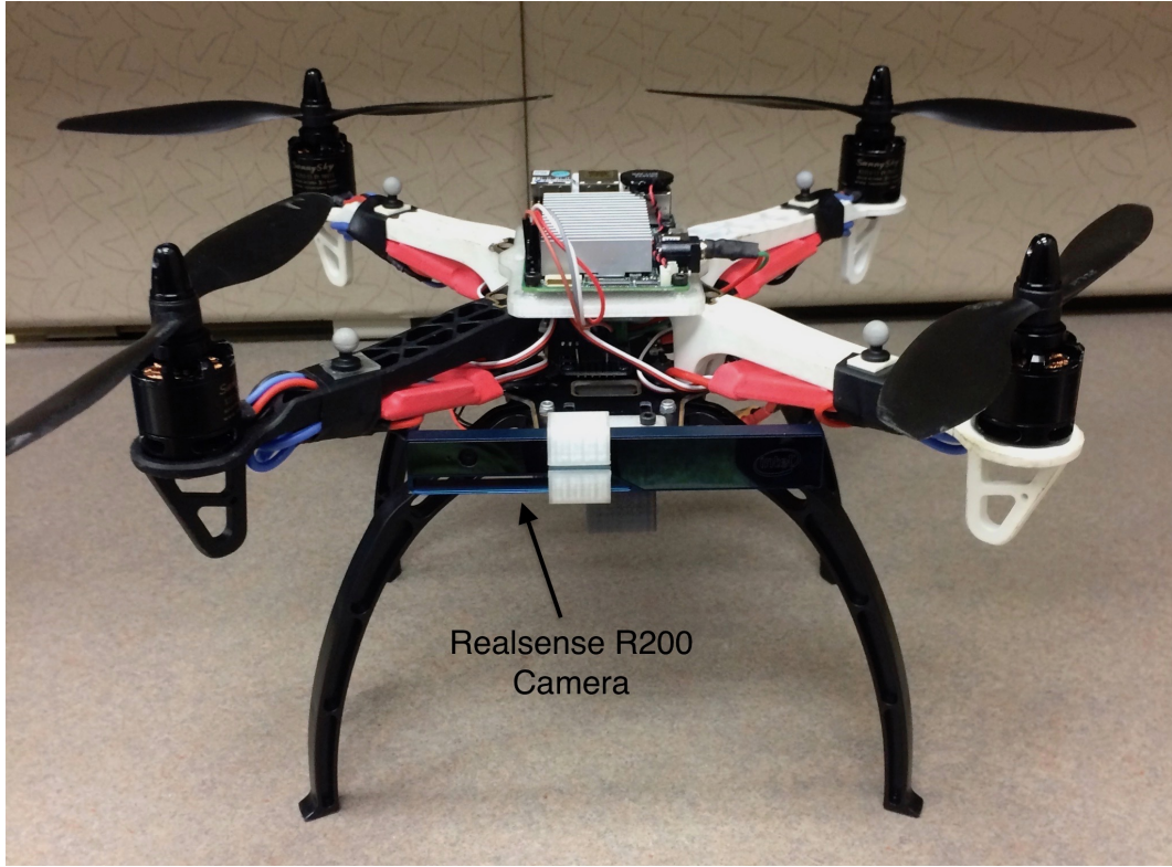
Figure 4.4: Front View of Fully Assembled Quadrotor. The Realsense camera is mounted to the front end of the bottom PCB.
