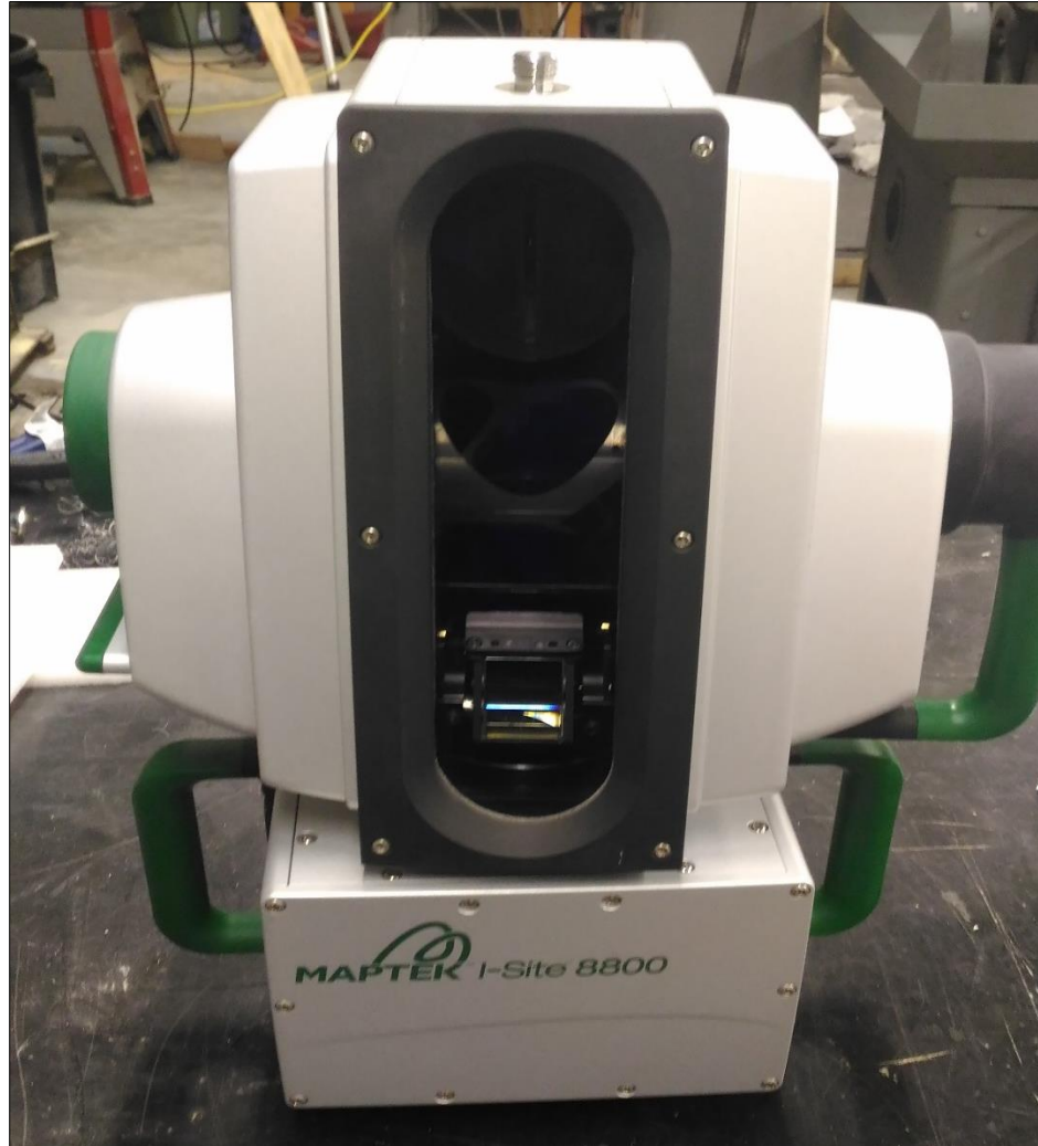
Figure 3-4: Maptek I-Site 8800 Scanner used to scan high-wall in field
