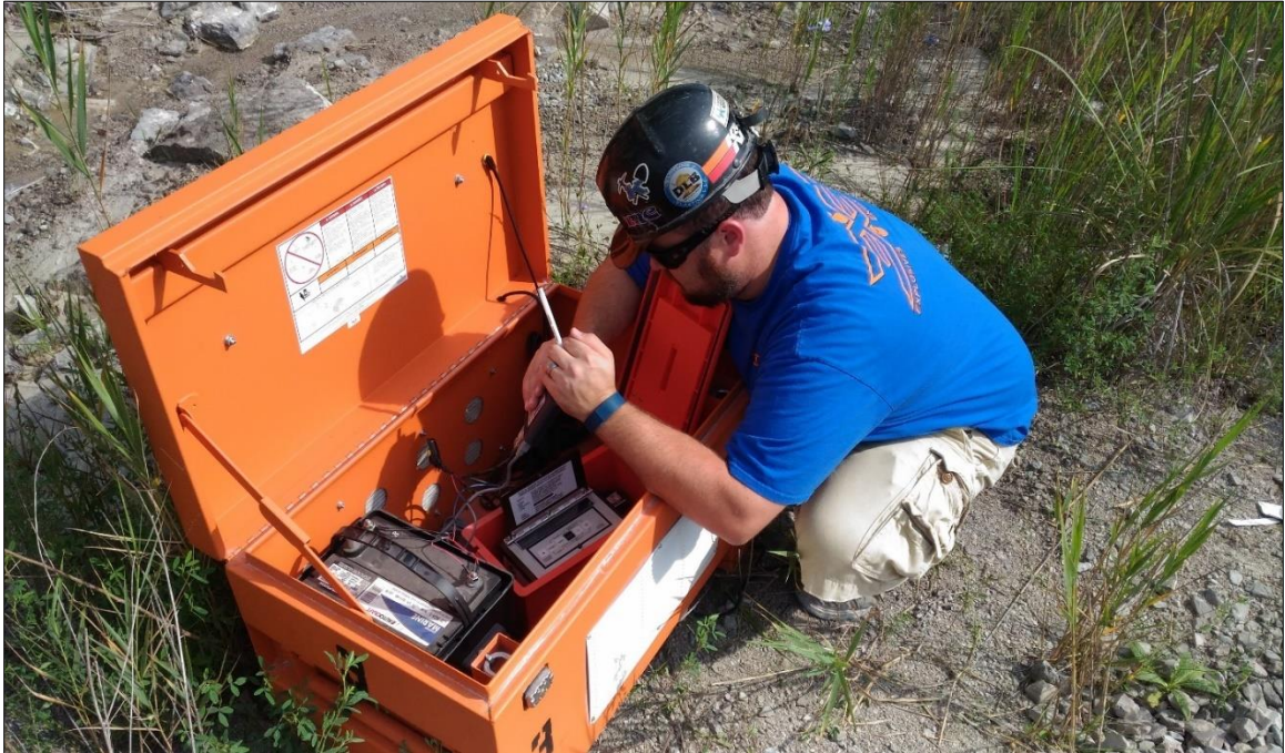
Figure 3-3: Setting up seismograph in field for data collection
