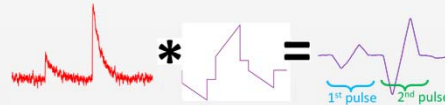
Example of a Double Trapezoidal Filter Convolution on a waveform with two pulses.
