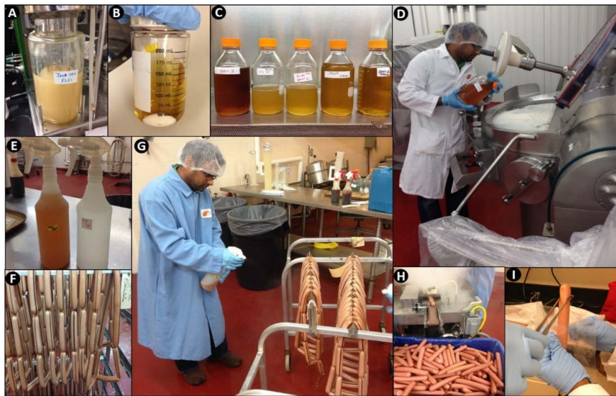
Figure 1. Manufacture of hotdogs for bacteriocin treatment. (A) Culturing microorganisms; (B) centrifugation of Bac + supernatants; (C) pasteurized Bac + CFS; (D) addition of Bac + CFS mixture to hotdog meat matrix (Trial #2); (E) spray bottles with pasteurized Bac + CFS; (F) pre-cooked hotdogs in casings; (G) spraying cooked hotdogs in casings with Bac + CFS mixture (Trial #2); (H) hotdogs after peeling; (I) addition of hotdogs to vacuum package bags for addition of Bac + CFS and the L. monocytogenes inoculum (Trials #3, #4, and #5).
