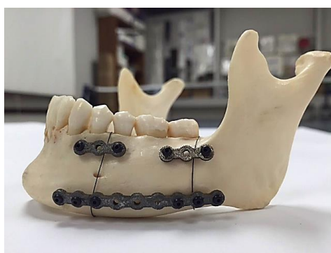
Figure 16. Reconstructed mandible using stiffness-matched, 3D printed, NiTi fixation devices.
