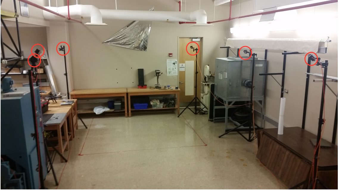
Figure 4.4: The 6 OptiTrack Prime 13 cameras are mounted on tripods, arranged in a circular configuration, pointed towards the test-flight volume, and angled slightly downward.
