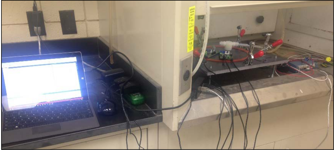
Figure 3-2. Sensors were calibrated in a fume hood while the program ran on a tablet PC.
