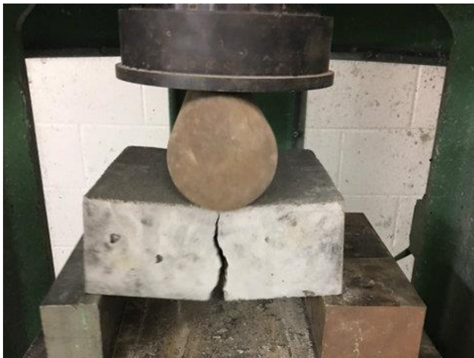
Figure 2 Breaking specimen for Healer/Sealer Testing
