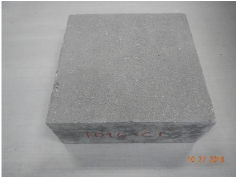
Figure 1 ICRI CSP3 Surface Preparation
