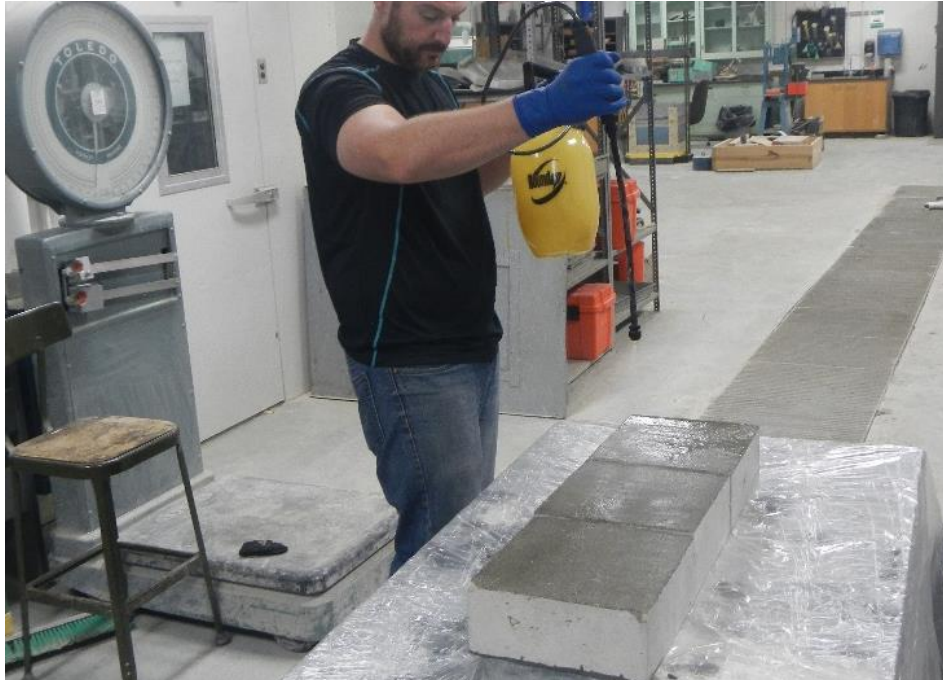
Figure 6 Application of Penetrating Sealer
