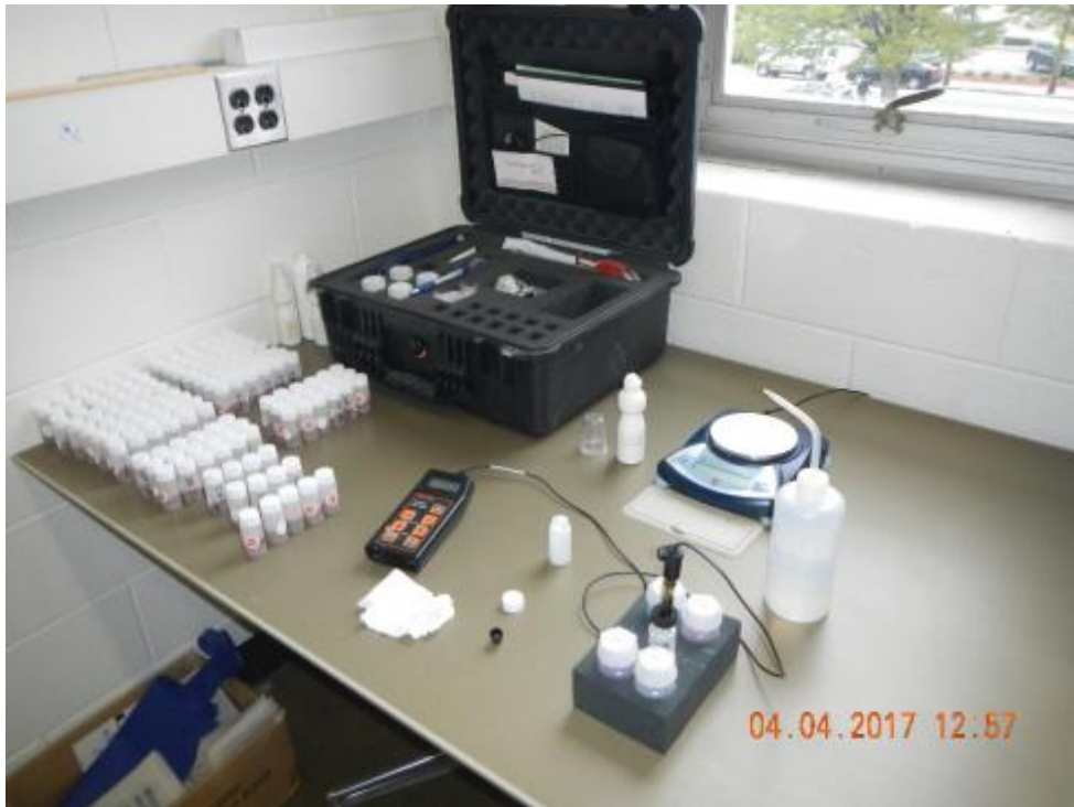
Figure 13 Germann Rapid Chloride Test (RCT)
