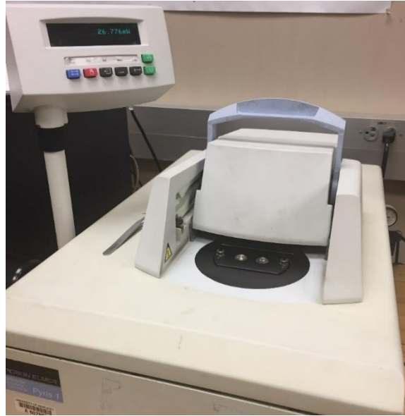
Figure 3.2: Perkin-Elmer Pyris 1 Differential Scanning Calorimeter to measure the stress free phase transformation temperatures.
