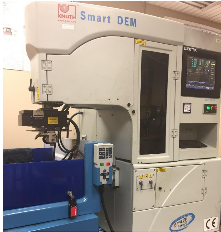
Figure 3.1: Electrical discharge machining (EDM) to cut specimens into desired shapes.
