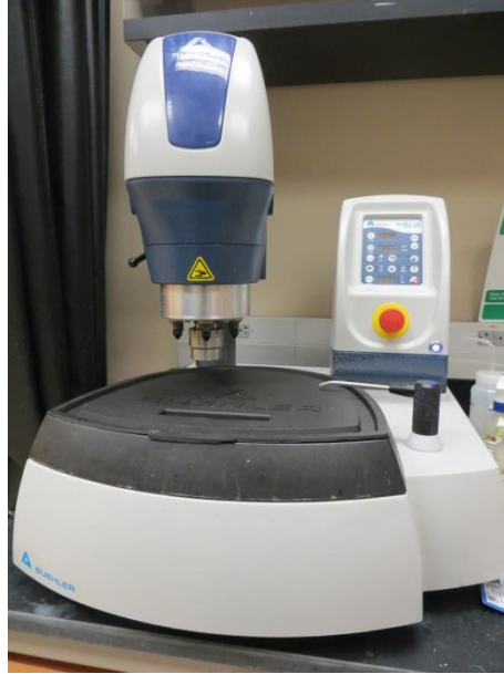
Figure 3.3: Buehler EcoMet 250 Grinder-Polisher (AutoMet 250 Power head) with chemical polishing.
