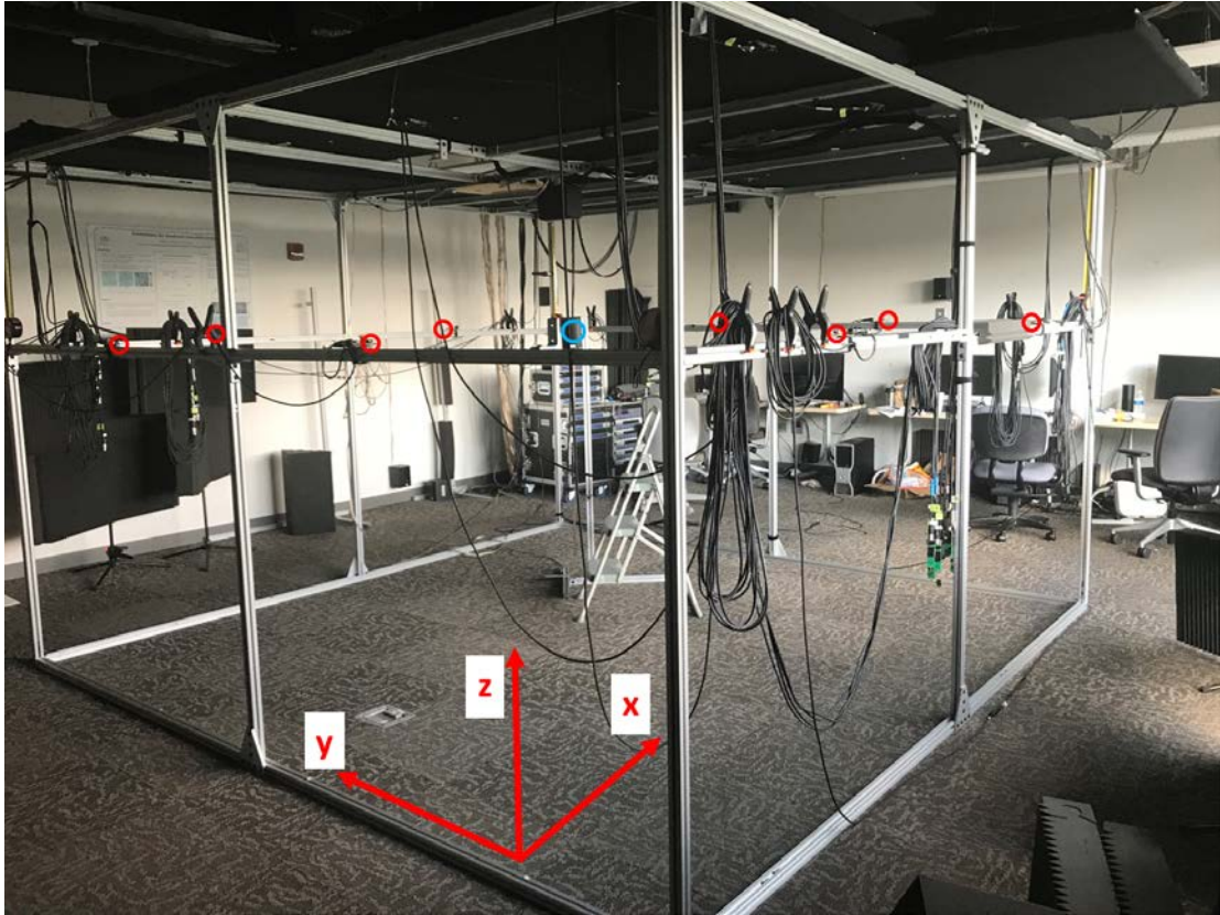
Figure 4.10 The lab environment where the experiment data collected. Red circles are microphones and blue circle is the speaker (sound source).
