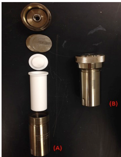
Figure 2.1 Schematic picture of hydrothermal reactor showing (A) showing components of hydrothermal reactor, stainless steel autoclave vessel and Teflon liner, and (B) the assembled hydrothermal reactor.
