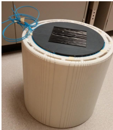
(a) Wire windings on the inner and outer shell.
