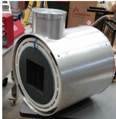
(b) The spin flipper inside the aluminum housing
