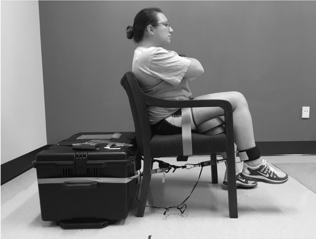
Figure 4.2: Seated isometric quadriceps strength testing set-up with a portable dynamometer.
