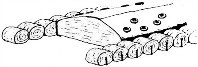
Figure 3. A temporary bunker silo using big round bales as sidewall retainers. Bales are set end wise to eliminate rolling and are blocked with a post at the outer end.
