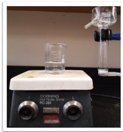
Figure 3. 5. Micro-flotation apparatus used for flotation tests.
