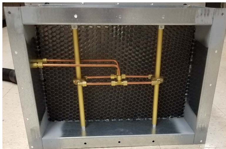
Figure 3.2: Inside of Dwyer STRA Airflow Measurement Station
