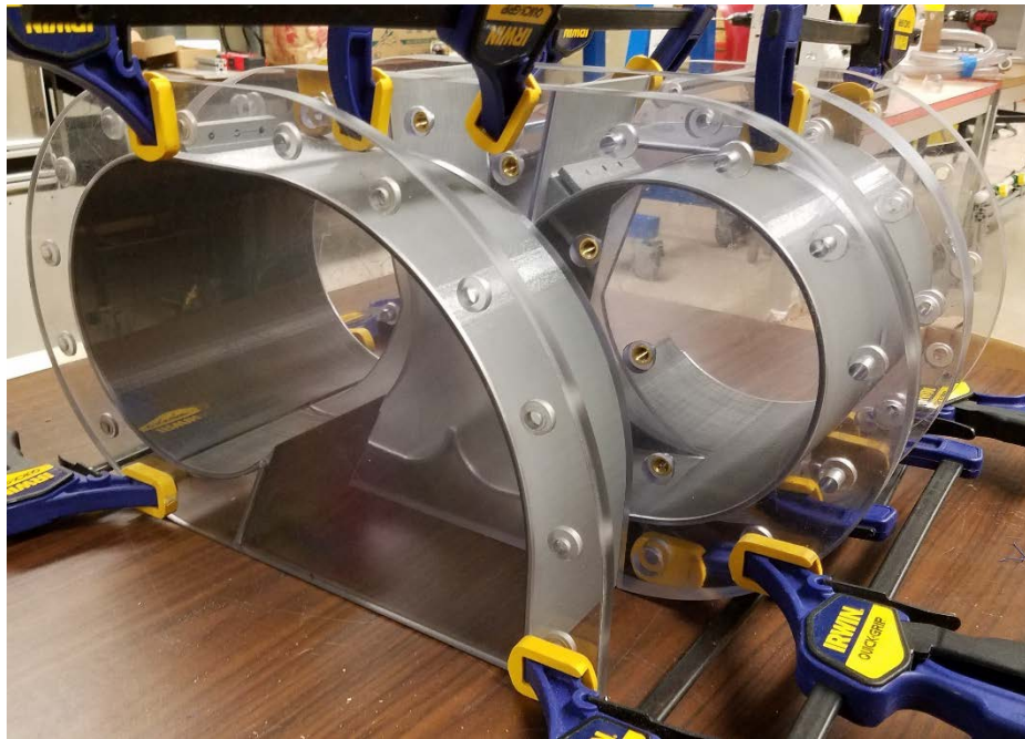
Figure 3.5: Vortecone in Early Stages of Construction
